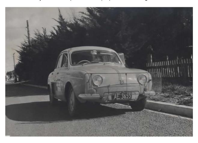
A pause at a control on the 72 Avery Motors trial. The car had recently done Gold star trials in the South Island. The device on the front was not a kangaroo catcher but a lightweight mesh screen for when following other cars on gravel roads needed some protection for the paintwork. The Perspex extension would allow for mounting a spotlight.
