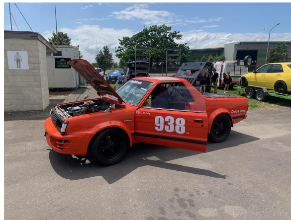
Subaru Ute with mid mounted engine and central driving position
