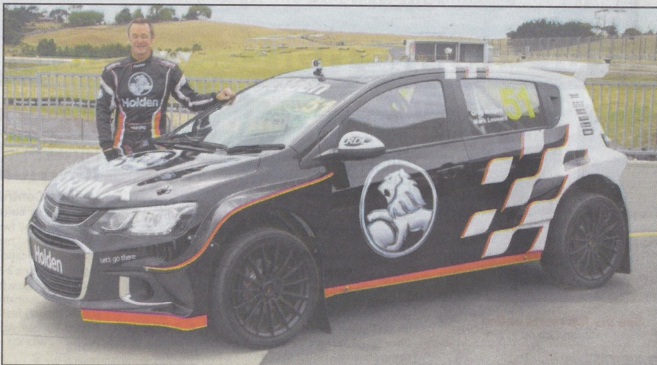
■ The Barina was stripped at RDL then the body and suspension fabrication was done at Force Motorsport. The car then went back to RDL for the balance of the build. A far cry from the road-going version, the AP4 is powered by a GM 2.0-litre four-cylinder that's been reduced to 1.8-litres; its Garrett GTX 2860 turbocharger boosting power to 350hp, and 500Nm of torque. It has a six-speed sequential gearbox.
