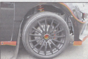
■ The Barina is all-wheel drive; brakes are Brembo calipers with AP cylinders, and a Tilton pedal box.
